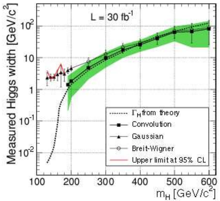
Measured Higgs boson width from a fit to the signal plus background distribution as a function of the Higgs mass
