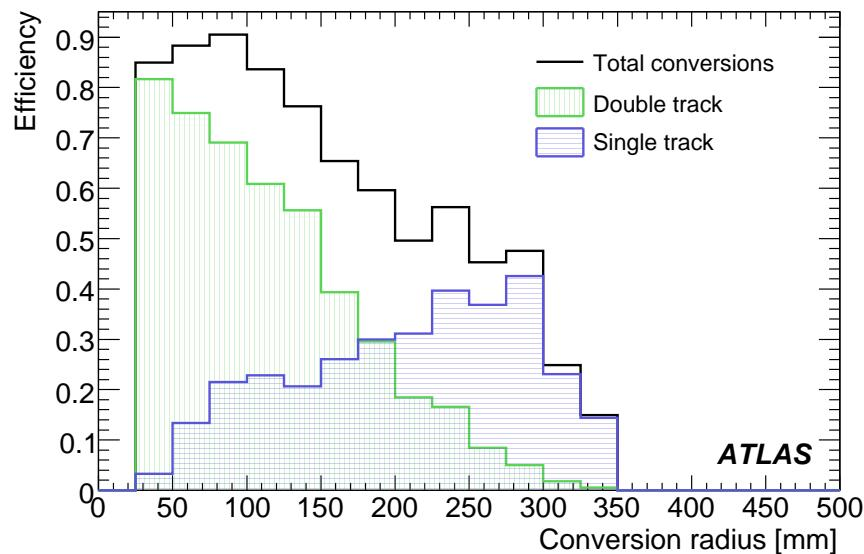
Efficiency of single-track and double-track conversion reconstruction as a function of the conversion radius
