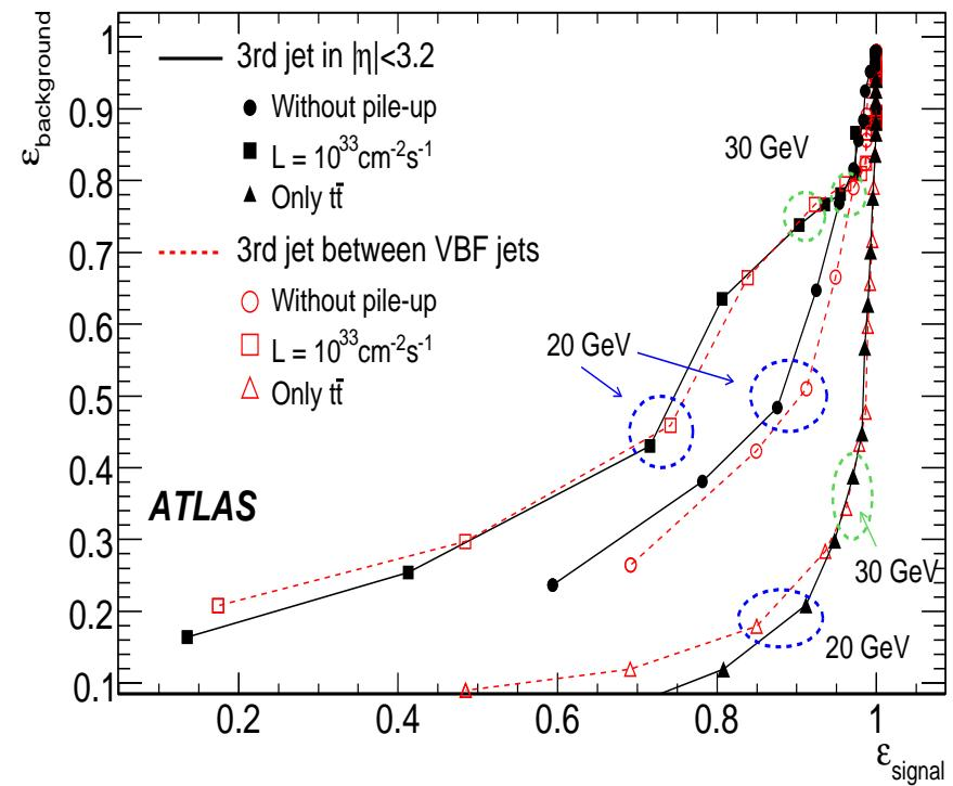
Background rejection versus signal sensitivity for the central jet veto with and without pile-up
