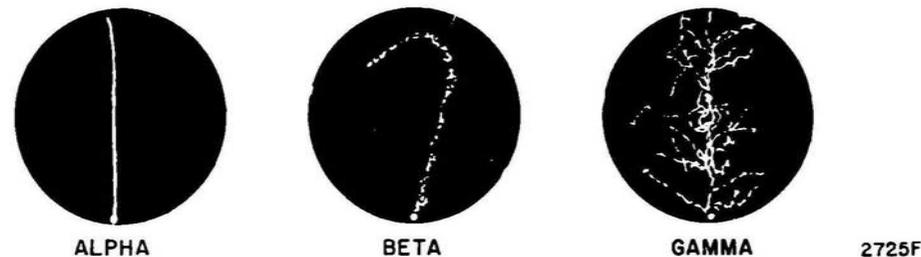
Figure 3-5. Cloud chamber photograph of alpha, beta, and gamma ray tracks. (J.B. Hoag: *Electron and Nuclear Physics*, courtesy D. Van Nostrand Co.) (H4)
