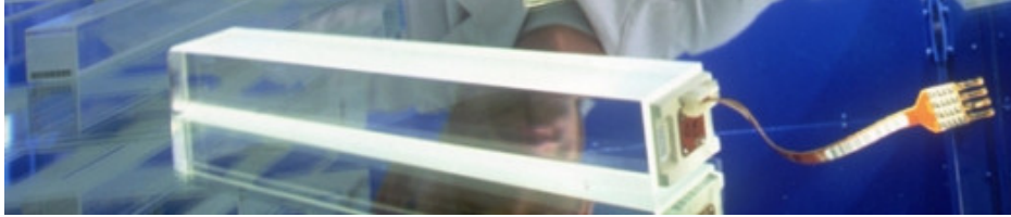
Figure 2.6.: A lead tungstate crystal, mated to the APDs. From [65].
